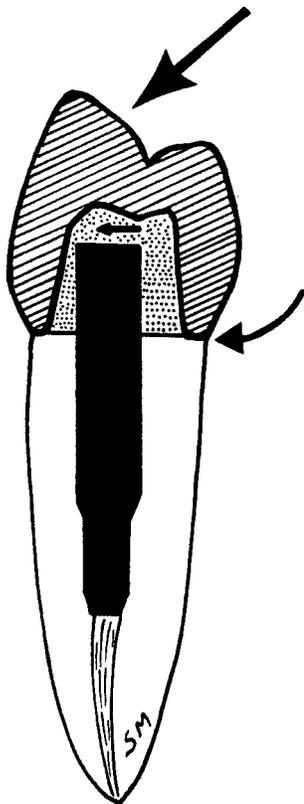
Fig. 7. Flexible post may allow micromovement of core (small arrow) under occlusal load (large arrow) when ferrule is small or absent with resultant fracture of cement seal at crown margin (curved arrow).
