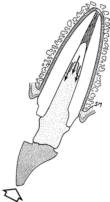
**Fig. 10.** Cement was placed on post only. As post is seated (*large arrow*) entrapped air within canal (*small arrows*) escapes through liquid cement, creating voids in cement film.
